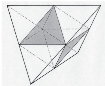
Above you can see how to construct a tetrahedron  $T_2$  with side 2 units using tetrahedrons  $T_1$  and a single octahedron  $O_1$ .
