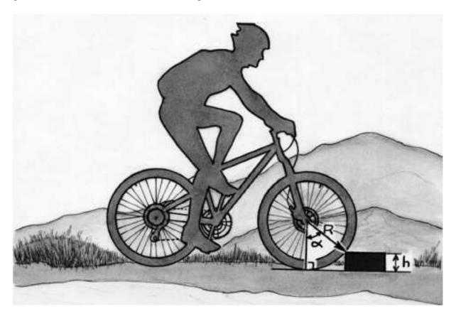
For an obstacle of height h = 8 inches, calculate the angle  $\alpha$  for each of the three wheel diameters.
